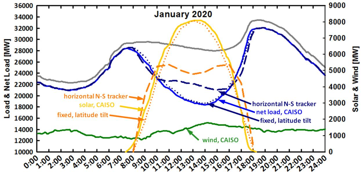
Figure 2. One example of the impact of tracking on the duck curve. Solar resource data is derived for Palmdale, CA in January.
