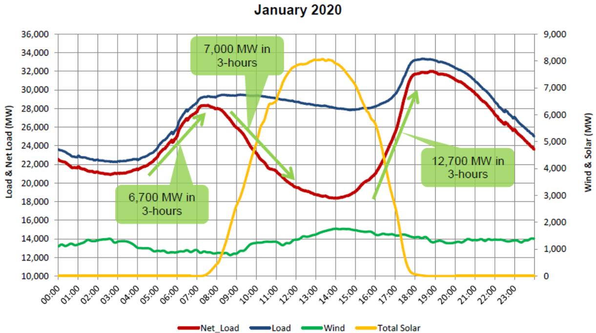
**Figure 6: Load, Wind, and Solar Profiles – Base Scenario**
